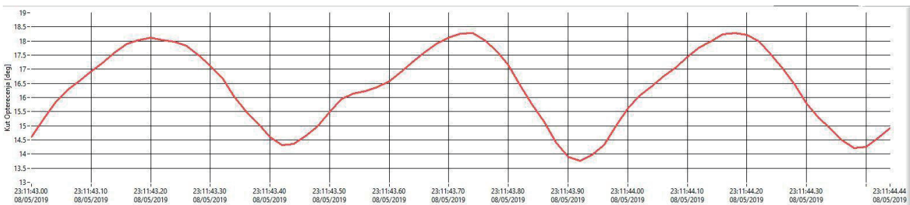
Fig. 7. Results of direct load angle measurement without geometrical imperfection correction
