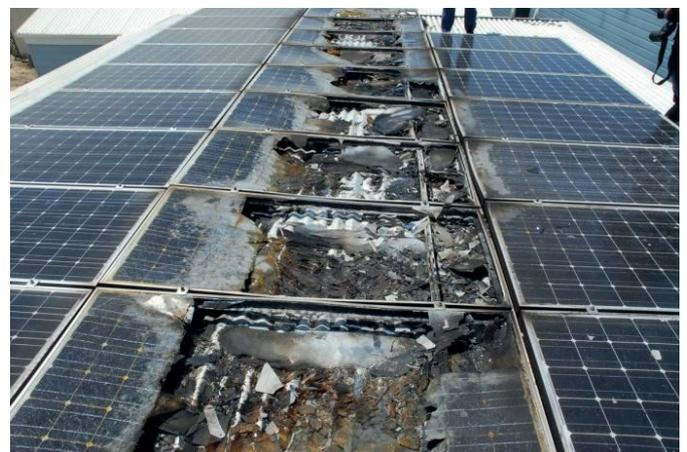
Figure 13. The consequence of fire on photovoltaic system, example [9]
