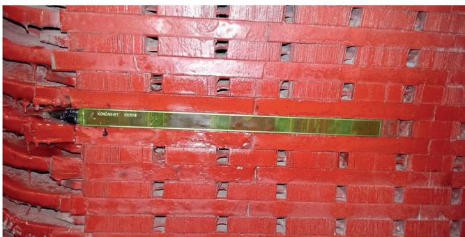
Figure 2. Measuring coil in PCB technique installed on the stator tooth
