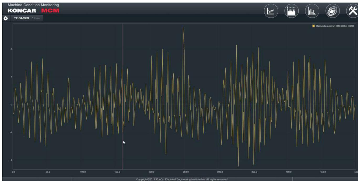
Figure 15. The induced voltage signal from measuring coil recorded by EMC system
