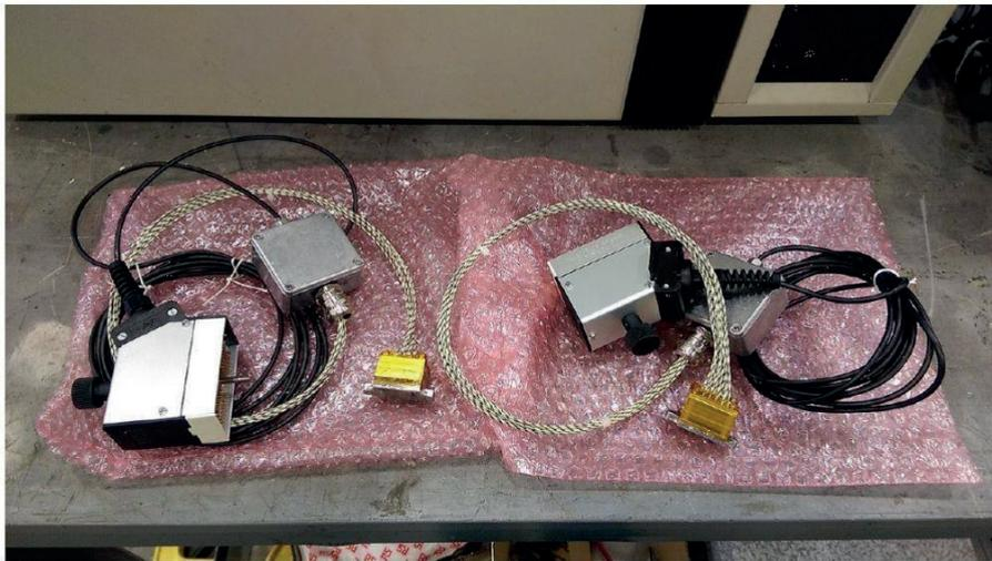
Figure 5: Two manufactured high temperature PA ultrasound probes using piezoelectric GaPO<sub>4</sub>
