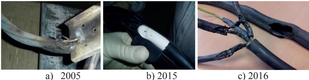
Figure 12: Failures due of LV power cables found with IR test
