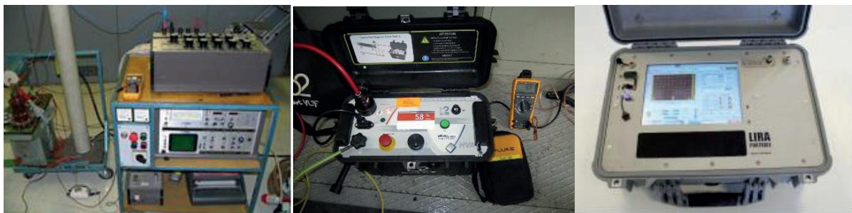
Figure 7: a)  $\tan \delta$  testing equipment with 50Hz and b) 0,1Hz and c) LIRA
