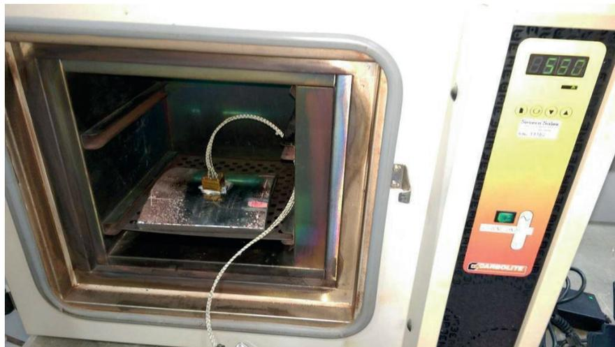
Figure 17: Phased array probe using GaPO<sub>4</sub> placed in an oven for characterisation at the target temperature of 580°C
