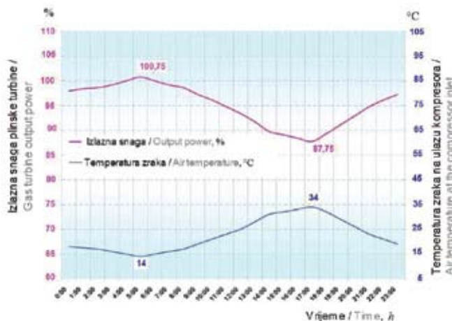
Slika 5 — Ovisnost izlazne snage plinske turbine o temperaturi zraka na usisu kompresora u tipičnom ljetnom danu Figure 5 — Dependency of gas turbine output power on the air temperature at the compressor inlet during a typical summer day
