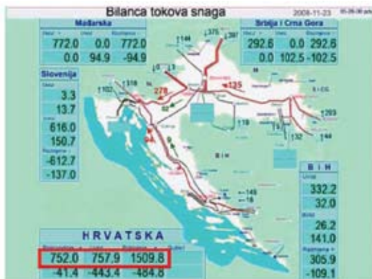
Slika 14 — Tokovi snaga u zimskom sušnom razdoblju (studen 2008. godine) [15] Figure 14 — Power flows during dry winter period (November 2008) [15]
