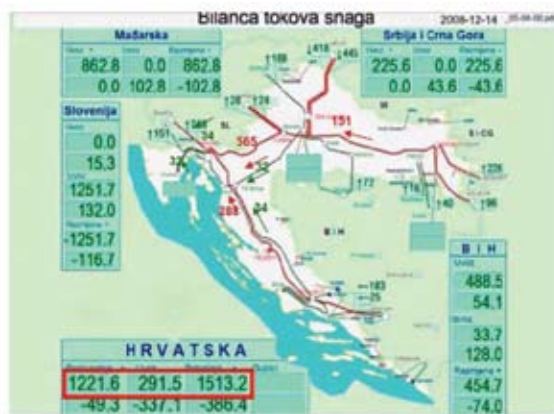
Slika 15 — Tokovi snaga u razdoblju povećanih dotoka zimi (prosinac 2008. godine) [15] Figure 15 — Power flows during favourable hydrology in winter period (December 2008) [15]
