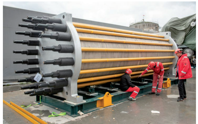
Fig.3. Hydrogen Pro Elektrolyser [12]
