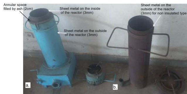
Fig. 4. The rice husk gasifier stove (a) the non-insulated type and (b) insulated type gasifier stoves
