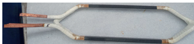
Fig. 1. Coil with shorten slot part – so-called “formette coil”
