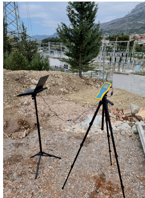
Fig. 5. Magnetic field measurement configuration in case of 110 kV overhead power line (fir tree mast)
