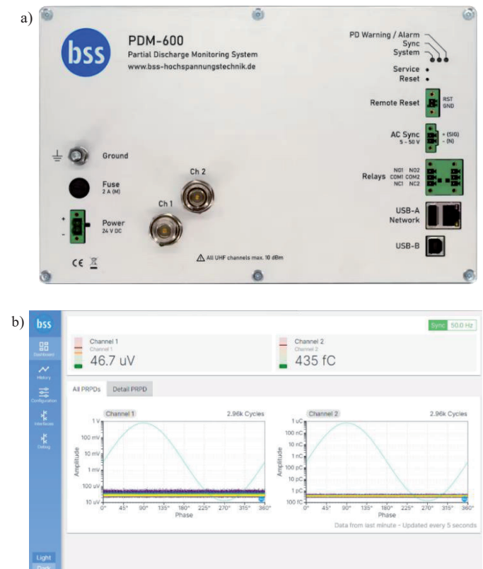
Fig. 2. a) PD monitoring system with 2 UHF channels [14]; b) web-based GUI showing live PD values and PRPDs
