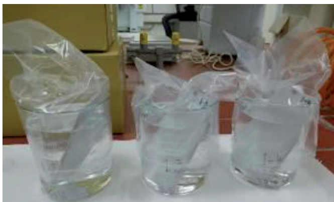
Fig. 10. Test coupons in immersion
