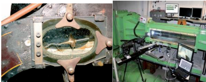
Figure 8. The test station of the propeller [10]
