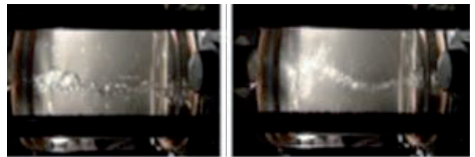
Figure 12. Travelling bubble type cavitation (left) Vortex rope cavitation (right) [36]
