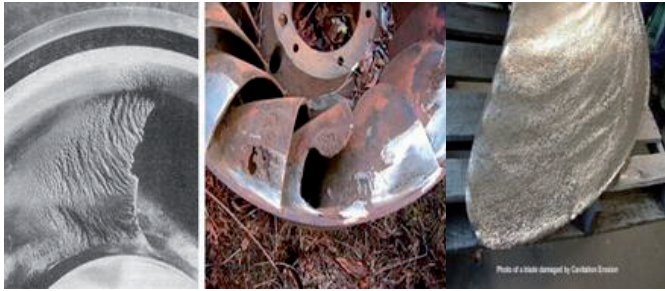
Figure 4. Cavitation erosion damage at pump and ships propeller [10, 11]
