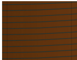
Figure 4 - Layers of copper (brown) and paper insulation (grey) during meshing process
