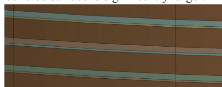
Figure 5 – Layers of copper discs (brown), paper insulation and spacer layer during meshing process
