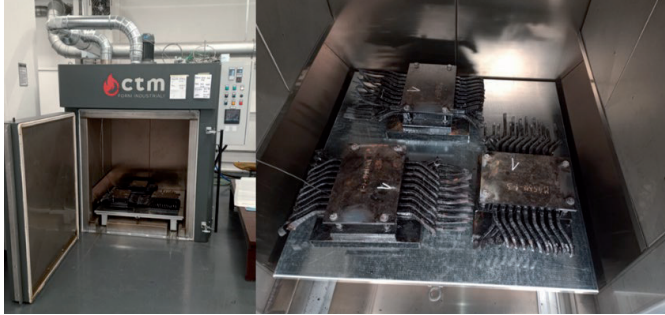
Fig. 4. Oven for thermal aging (left) and test objects inside of the oven (right)
