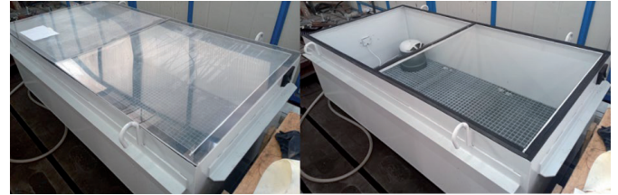
Fig. 6. Condensation chamber with (left) and without (right) cover
