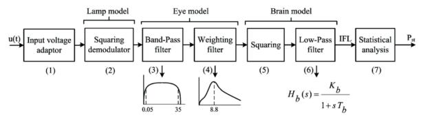
Figure 2. Block diagam of a standard IEC flickermeter [11]
