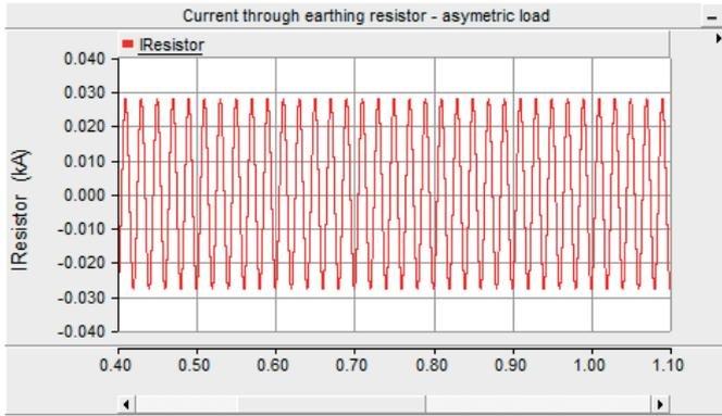
Figure 13: Current through earthing resistor of artificial ground point — highly asymmetrical loads
