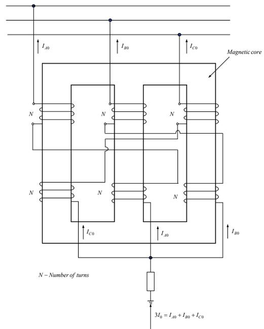
Figure 2: Winding connections of the zigzag grounding transformer
