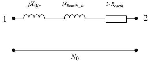
Figure 6: Zero sequence connection of grounding transformer in combination with short circuit limiting resistor
