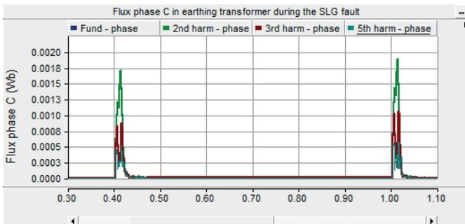
Figure 22: Detailed view of flux oscillation by harmonics during the SLG fault
