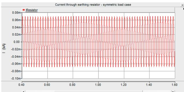
Figure 11: Current through earthing resistor — normal operation of MV power network
