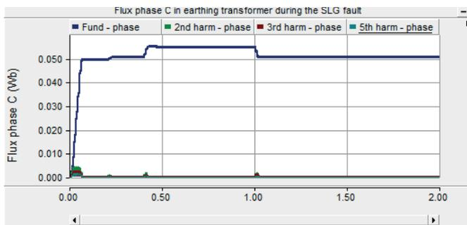
Figure 21: Harmonic decomposition of magnetic flux of grounding transformer
