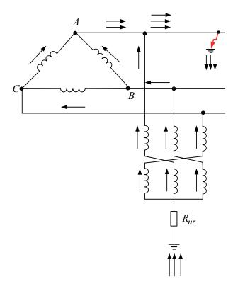
Figure 3: SLG short-circuit distribution inside the grounding transformer
