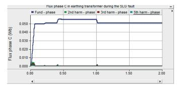
Figure 21: Harmonic decomposition of magnetic flux of grounding transformer
