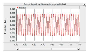
Figure 13: Current through earthing resistor of artifficial ground point — higly asymmetrical loads
