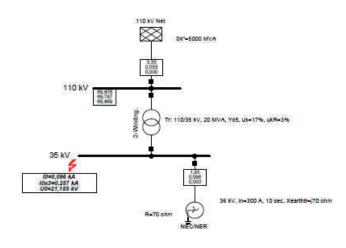
Figure 8: Computer simulation - SLG fault on 35 kV busbars
