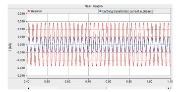
Figure 15: Earthing resistor current of artifficial grounding point connection and grounding transfomer phase B current
