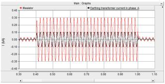
Figure 18: Earthing resistor current of artificial grounding point connection and grounding transfomer phase A current - SLG fault
