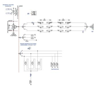
Figure 12: Simulation model of 35 kV power network with grounding transformer neutral point connection — asymmetrical loads
