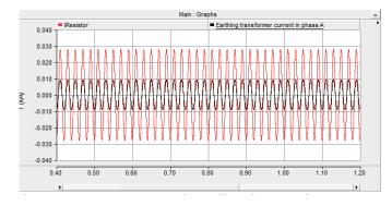
Figure 14: Earthing resistor current of artifficial grounding point connection and grounding transfomer phase A current
