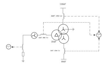
Figure 4: Protection principle of characteristic feeding transformer
