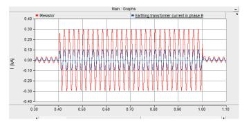
Figure 19 Earthing resistor current of artificial grounding point connection and grounding transfomer phase B current — SLG fault
