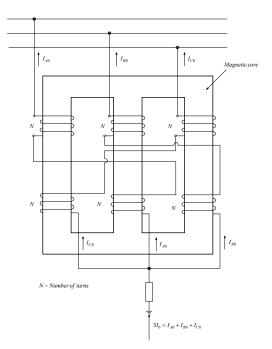
Figure 2: Winding connections of the zigzag grounding transformer
