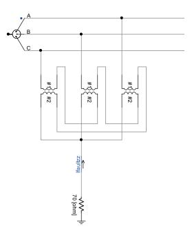
Figure 9: Model of grounding zigzag transformer for artifficial ground point
