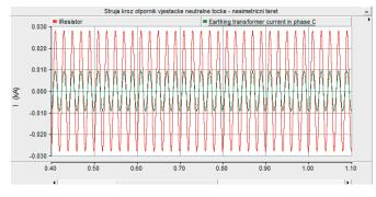
Figure 16: Earthing resistor current of artifficial grounding point connection and grounding transfomer phase C current
