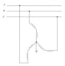
Figure 1: Principle of zigzag earthing transformer connection
