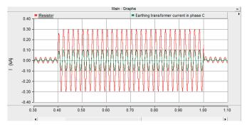
Figure 20 Earthing resistor current of artificial grounding point connection and grounding transfomer phase C current — SLG fault
