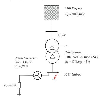
Figure 5: Typical MV power network with zigzag grounding transformer for example of short–circuit calculation with symmetrical components
